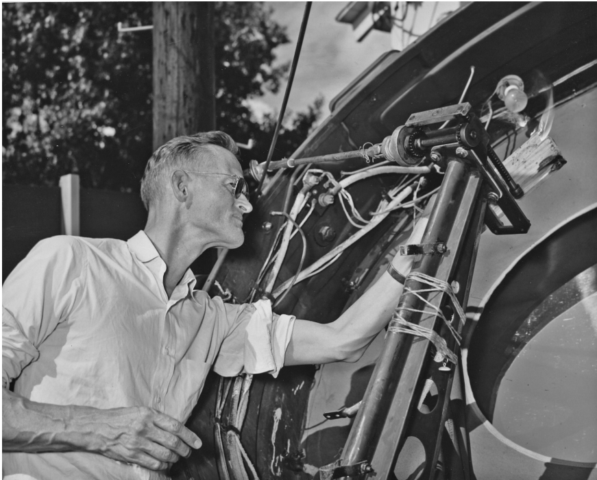
Fig. 1: Simulating atomic heat: Konrad Büttner experimenting with his custom-made solar reflector at the Air Force School of Aviation Medicine, early 1950s.
